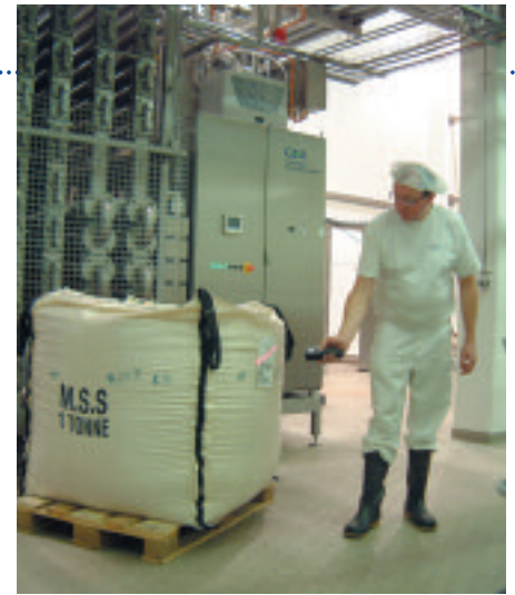
Additions of powder are recorded via mobile barcode scanners for batch tracing and product management
