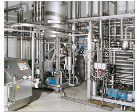
Heating plant / deaeration / homogenisation
